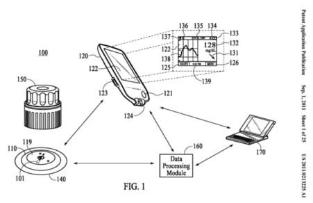
22.4. The Court notes that Bernstein discloses a monitoring system with an analyte sensor (101), an on-body electronics unit (110) configured to store monitored analyte-related data received from the analyte sensor and a display device (120).
