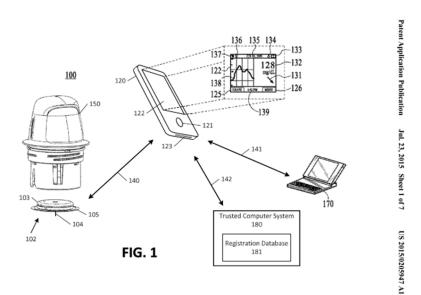
Figure 1 (D1) shows an analyte monitoring system, comprising:
